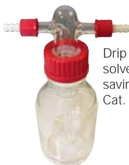
Drip Catcher for taking solvent prior to the pump saving expensive water.
