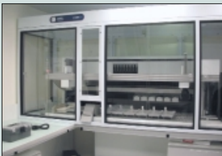
Bench mounted system including chute for used tips
