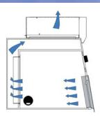
The electronic control system continually monitors the air flow measured by an anemometer located in the aperture at the front of the enclosure and automatically responds to any significant airflow disturbance within the laboratory.
