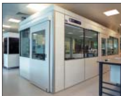
Environmentally controlled room for a mass spectrometer system
