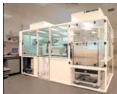
Robotic enclosure for the containment of a high throughput screening system
