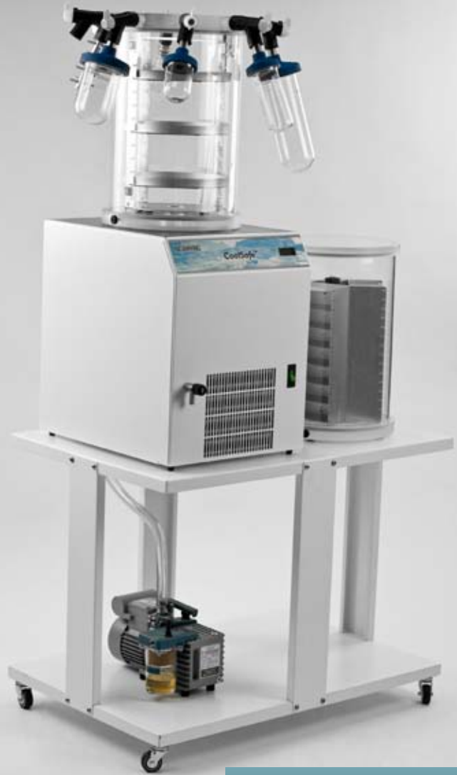
Chamber CC300-8V with shelves and manifold combined.
