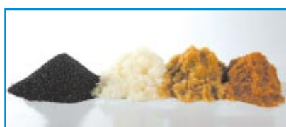
High grade materials are a vital aspect for highest quality. From left to right: Activated carbon, anions-, mixed bed- and cationexchange resins.
